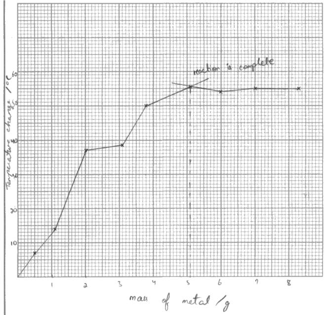
(ii) Determine the mass of metal **M** that reacts exactly with 50.0 cm<sup>3</sup> of 1.35 mol dm<sup>-3</sup> copper(II) sulfate by drawing appropriate best-fit straight lines. You **must** show your working on the graph.
